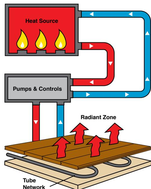
This diagram is a conceptual diagram of the basics of how radiant heat works. It is not a working diagram for installation purposes.
