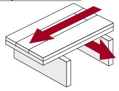
When installing the flooring in the same direction of the joists, a second layer of plywood is required to stiffen sub floor. Subfloor must be sheeted with  $\frac{1}{2}$ " (15/32", 14mm) CD exposure 1 plywood sub floor panels. Use same method as attaching to solid board sub flooring.
